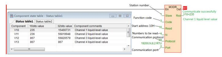
The host PLC reads the 4-channel liquid level values of SMC-AD04EN by Modbus read instruction MODR, the start address is 10H (hexadecimal), that is, the decimal value is 16. When the communication is successful, M0 is ON, the liquid level values which are read back will be stored in V0-3, V0=235, indicating that the actual temperature of the first channel is 0.235m, the same as V3=867, indicating that the actual temperature of the fourth channel is 0.867m.
