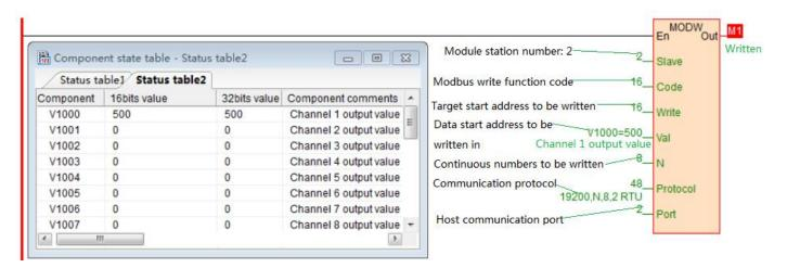
Host PLC writes the 8-channel analog output values of SMC-DA08EN by Modbus write instruction MODW, the start address is 10H (hexadecimal), that is, the decimal value is 16. When writing successfully, M1 is ON, the 8-channel values which will be written into are stored in V1000-1007.
