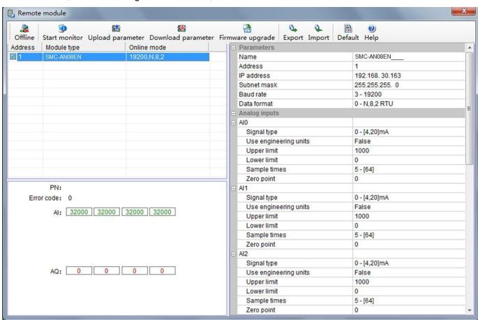
We can change the module name, address, IP, subnet mask, baud rate, data format and other communication parameters in the communication parameter area.
