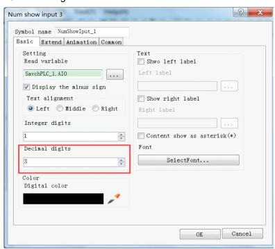
So that when the PLC read Al0 value, Al0=1234, that is the actual value of 1.234Mpa, there is no need to have data processing in PLC and configuration, only set the 3 decimal places on the numerical display primitive, then it will be automatically reduced by 1000 times, displaying value of 1.234, that is the actual value of 1.234Mpa.
