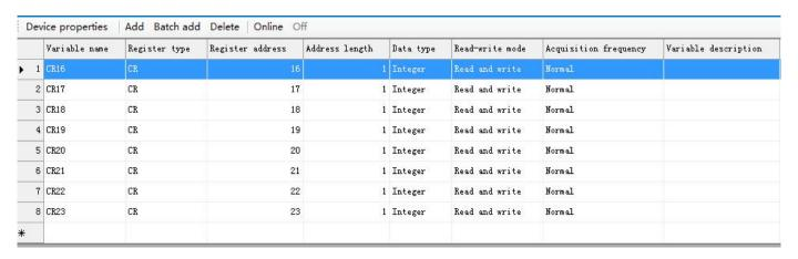
Then set up the screen, we can use the display primitives to bind the corresponding channel variable values. If you need to display the decimal places, it can set the corresponding decimal places on the display primitive. As shown below:
