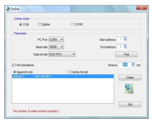
If there is only one machine connected with 485 line, then check "stand-alone search"; if there are more than one, then remove the button of "stand-alone search", and set the start address and end address, so that all the machines connected with 485 line can be found and achieve parameter configuration.
