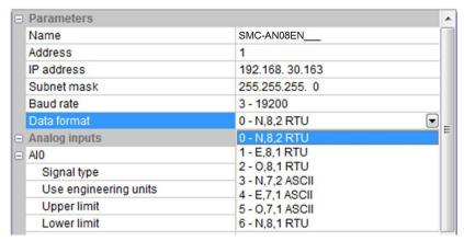
In the external analog input area, we can set the signal type of each channel, choose whether to use engineering value or not, the upper and lower limits of engineering value(it can be set if you check the use of engineering value), sampling times and zero correction.
