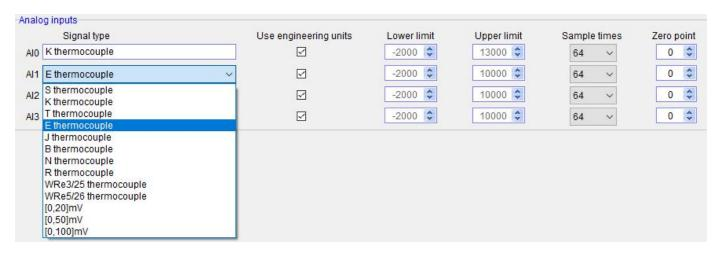
In this way, after configuration, as long as connect the K-type thermocouple to channel 1, then directly read Al0 register value, Al0 = 123, that is the actual value of 12.3  $^{\circ}$ C. In the same way, connect E-type thermocouple to channel 2, read Al2 value, such as Al2 = 3456, that is the actual value of 345.6  $^{\circ}$ C.
