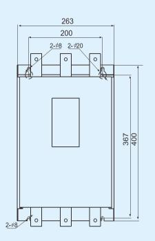
• External & installation dimensions for 250A-450A (Unit: mm)
