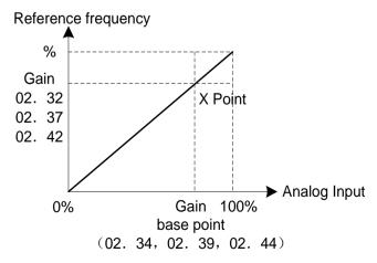
Note:To input bipolar analog voltage (0 to ±10 DC) to terminals AVI and AUI, set 02. 35 and 02. 45 data to "0." Setting 02. 35 and 02. 45 data to "1" enables the voltage range from DC 0 to +10 VDC and interprets the negative polarity input from DC0 to -10 V as 0 V.
