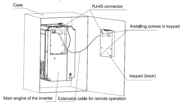
Figure 2.11 Install keypad in the disc
