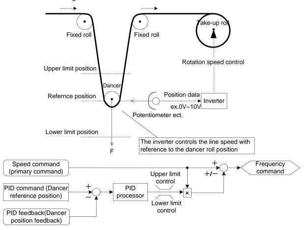
Using this parameter enables switching between normal and inverse operations against the PID control output, so you can specify an increase/decrease of the motor rotating speed to the difference or error component (between the commanded (input) and feedback amounts), making it possible to apply the inverter to air conditioners.
