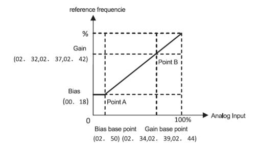
Note:terminals AVI and ACI (if the sum of AVI+ACI is enabled), the bias and gain are independently applied to each of the voltage and current inputs given to terminals AVI+ACI, and the sum of the two values is applied as the reference frequency.
