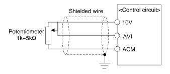
Figure 2.5 Shielded cable connection figure
