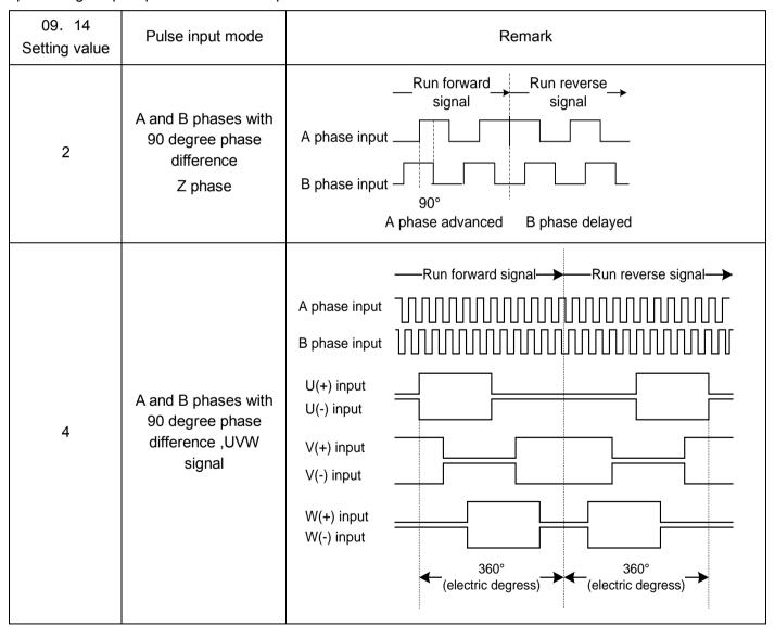
Note: When changing the setting of parameter 09. 14, it requires to do a adjustment again for the magnetic pole postion sensor compensation (03. 95). The inverter can adjust automatically via auto-tuning.
