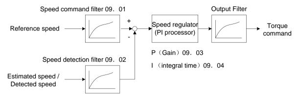
Block diagram of the speed control sequence
