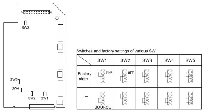
Figure 2.10 The locations of various switches on control circuit board
