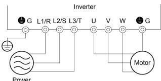
Fig 4.1 Connection Diagram of Main Circuit Terminals
