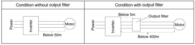
When there is an output filter, please ensure that the total length of wiring is within 400m (within 100m when vector controls)
