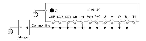
Figure 8.2 Wiring diagram of Main Circuit Terminal for Megger Test
