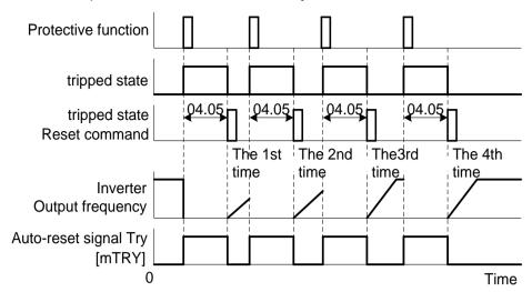
· Under the circumstance of output alarm when it is restarted for more than 3 times (04. 04=3)
