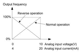
Tips:The normal/inverse switching operation is useful for air-conditioners that require switching between cooling and heating. In cooling, the speed of the fan motor (output frequency of the inverter) is increased to lower the temperature. In heating, it is reduced to lower the temperature. This switching is realized by this [mIVS] terminal command
