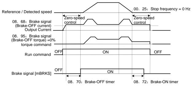
Note ·If the zero speed control is enabled, set 08. 95 (Brake-OFF torque) at 0%.
