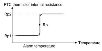
Suppose that the internal resistance of the PTC thermistor at the alarm temperature is Rp, the detection level (voltage)  $V_{V2}$  is calculated by the expression below. Set the result  $V_{V2}$  to function parameter 04. 27.
