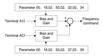
In the case of unipolar input (terminal AVI(with 02.35 = 1, terminal ACI, terminal AUI with 0.245 = 1)
