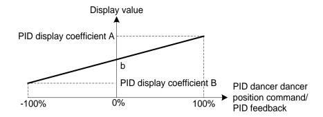
If the sensor output is unipolar, the PID dancer control operates within the range from 0 to +100%, so virtually specify the value at -100% as coefficient B.
