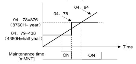
2)(Preset startup count for maintenance (M1)) 04. 79 specifies the number of inverter startup times to determine the next maintenance timing. When the count of the startup counter for motor 1 (04. 44) reaches the number specified by 04. 79 (Preset startup count for maintenance (M1)), the inverter outputs the maintenance timer signal [mMNT] to remind the user of the need of system maintenance.
