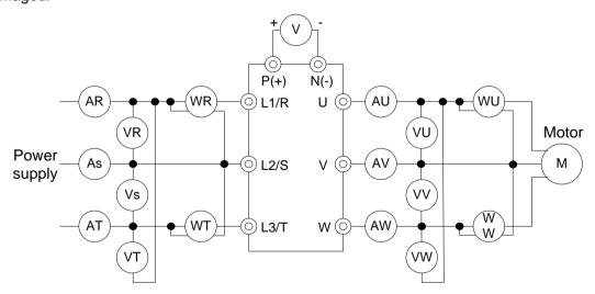
Figure 8.1 Wiring diagram of meters
