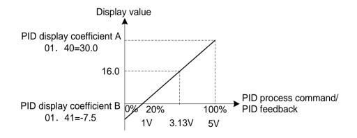
■Display coefficients for PID dancer position command and its feedback (08. 01=3)
