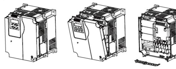
Figure 2.2 Removal of surface cover and cable lead-in plate (case of S5100-4T5.5G ~ 22G)
