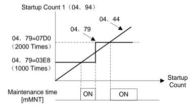
To enable this function, assign the maintenance timer signal [mMNT] to one of the digital output terminals (function parameter data = 84).
