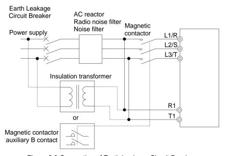
Figure 2.3 Connection of Earth Leakage Circuit Breaker
