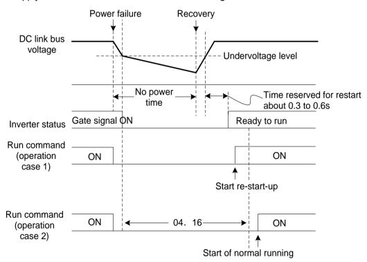
If 04. 16 (Allowable momentary power failure time) is set to "999," restart will take place until the DC link bus voltage drops down to the allowable voltage for restart after a momentary power failure (50 V for 230 V series and 100 V for 400 V series). If the DC link bus voltage drops below the allowable voltage, the inverter recognizes that the power has been shut down so that it does not restart but starts (normal starting)
