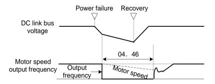
Notes: To use auto search for idling motor speed, it is necessary to tune the inverter beforehand.
