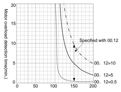
(Actual output current value/Overlead detection level) X 100%
