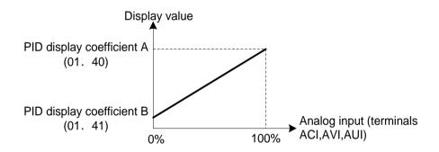
To set up the analog input monitor, use function parameters 01. 61 to 01. 63. Use 01. 43 to choose the item to be displayed.
