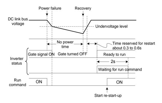
Note: When the power is restored, the inverter will wait 2 seconds for input of a run command. However, if the allowable momentary power failure time (04. 16) elapses after the power failure was recognized, even within the 2 seconds, the restart time for a run command is canceled. The inverter will start operation in the normal starting sequence.
