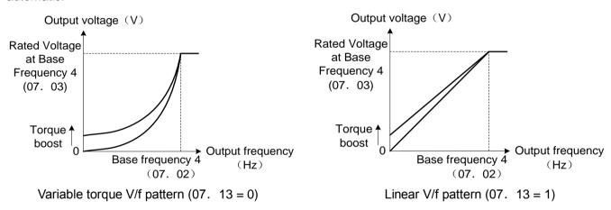
Tips: When the variable torque V/f pattern is selected (00. 37= 0 or 3), the output voltage may be low at a low frequency zone, resulting in insufficient output torque, depending on the characteristics of the motor and load. In such a case, it is recommended to increase the output voltage at the low frequency zone using the non-linear V/f pattern.
