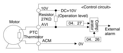
Note: When using the terminal AUI for PTC/NTC thermistor input, also turn SW5 on the control board to the PTC/NTC side.
