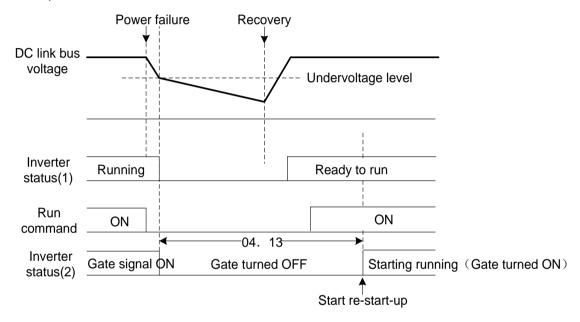
Note:04. 13 (Restart mode after momentary power failure -- Restart time) also applies to the switching operation between line and inverter (Parameters 01. 01~01. 09).
