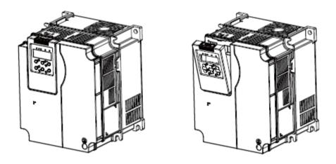
Figure 2.12 Removal of keypad
