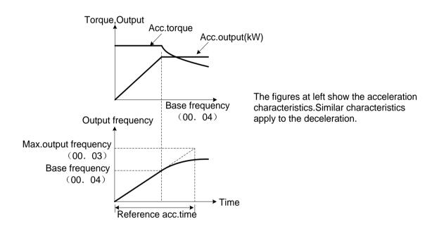
Note: If you choose S-curve acceleration/deceleration or curvilinear acceleration/deceleration in Acceleration/
