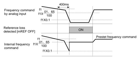
In the diagram above, f1 is the level of the analog frequency command sampled at any given time. The sampling is repeated at regular intervals to continually monitor the wiring connection of the analog frequency command.
