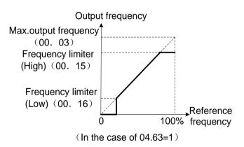
Notes:When you change the frequency limiter (High) (00. 15) in order to raise the reference frequency, be sure to change the maximum frequency (00. 03) accordingly.
