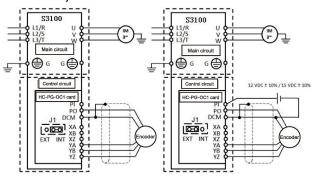
Used the inverter internal power wiring diagram (J1 jumper in the INT position)
